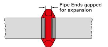
For thermal contraction with flexible couplings, the pipe ends at each joint should be fully butted. The system can then be anchored in place to prevent the pipe ends from opening up to the maximum end gap when pressurized.
