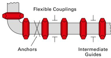
3. Design the system with flexible couplings utilizing the expansion/contraction capabilities of these products. The following example illustrates this method:
